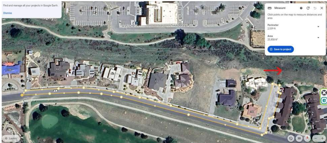
5/29/2023 imagery with impervious area delineated and erosion due to stormwater point discharge indicated by red arrow.
