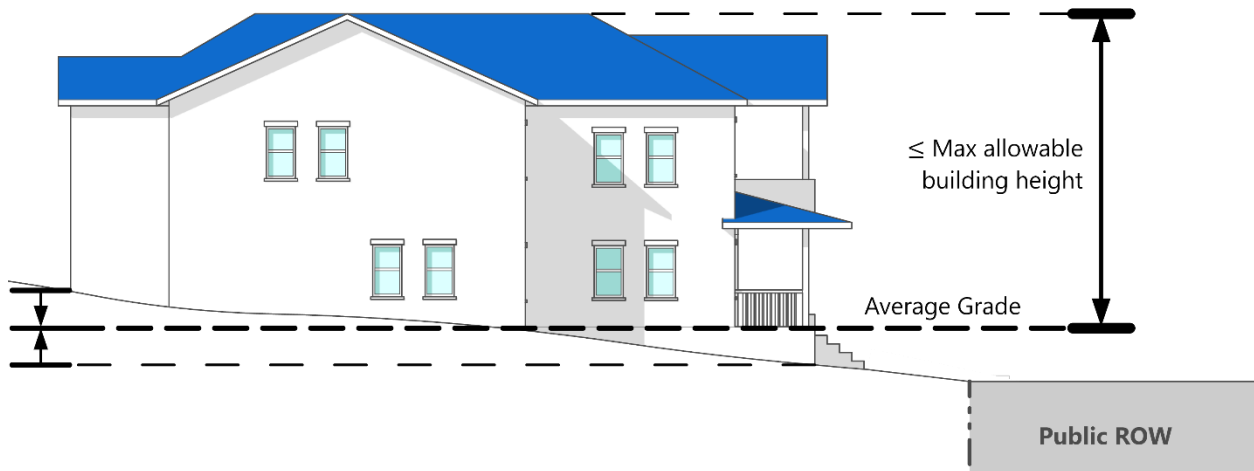
Figure 2-3: Measurement of Building Height on Uneven Lot
